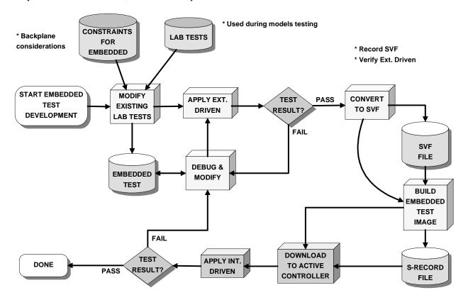
**Figure 3- Embedded Test Process Flow**
