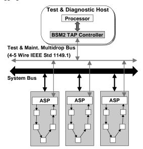
Figure 2 – Multidrop scan channel
