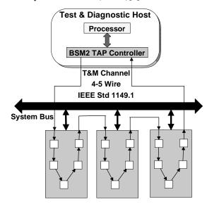
Figure 1 – Serially connected scan chain
